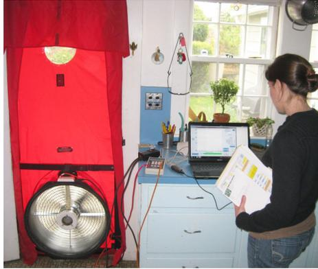
basement and attic closed) was 2258 CFM 50, but was 2743 CFM 50 with the basement open (which is closer to post-retrofit conditions). The post-retrofit measurement (including basement and attic) was 236 CFM 50. With the air barrier boundary establishing the total volume, this is approximately equivalent to 0.6 ACH 50.
